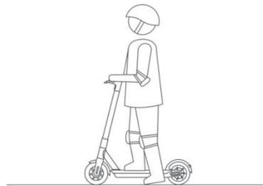
2. With an initial speed no lower than 2.5mph and press the throttle to start the scooter, sport mode with maximum speed of 15.5mph, and it also can be customized for local customer' s actual speed requirement. To turn, shift your body weight and turn the handle slightly.
